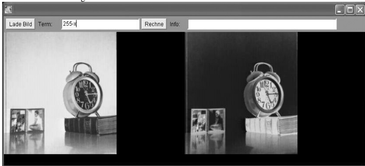
Fig 4: An Applet to transform the brightness of pixels according to a function
